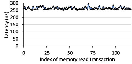
Fig. 2. Global memory access latency on the GPU ( S=2\text{KB} , W=16\text{MB} )
